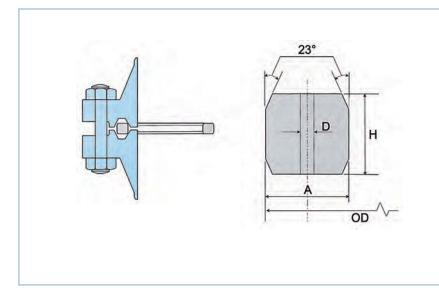
NOTE 1: Radius of the ring shall be 8% to 12% of the ring height 'H'.
