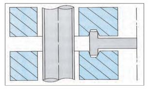
Section through Blind Ring Type Joint
