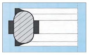
Section through a Rubber Ring Joint
